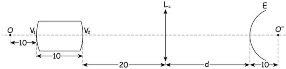
$$n_1 \left( \frac{1}{r_1} - \frac{1}{S_1} \right) = n'_1 \left( \frac{1}{r_1} - \frac{1}{S'_1} \right) \Rightarrow 1 \left( \frac{1}{20} - \frac{1}{-10} \right) = 1.5 \left( \frac{1}{20} - \frac{1}{S'_1} \right) \Rightarrow S'_1 = -20 \text{ cm}$$
